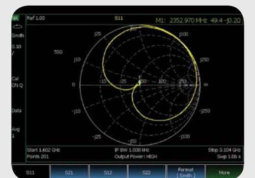
Impedance tuning using the Smith chart
